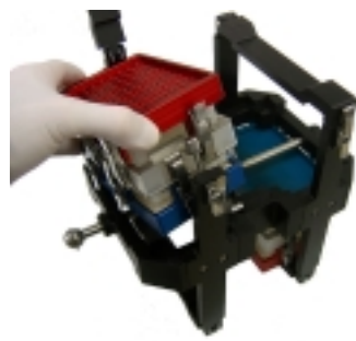
2. Place sealed reactor blocks in rotator.
