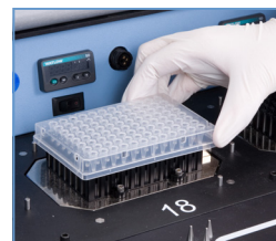
Figure 5. Add sample plate.
