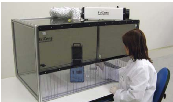
The NoZone® WS Workspace maintains ozone levels below 5 ppb when washing and drying microarrays.
