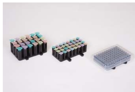
Three blocks are available for 0.2, 0.6 or 1.5 ml tubes.
