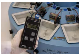
Hybridization and wash temperatures are precisely controlled and can be independently validated.
