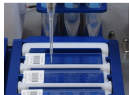
The robot dispenses metaphase cells for G-banding in up to 3 locations per slide.
