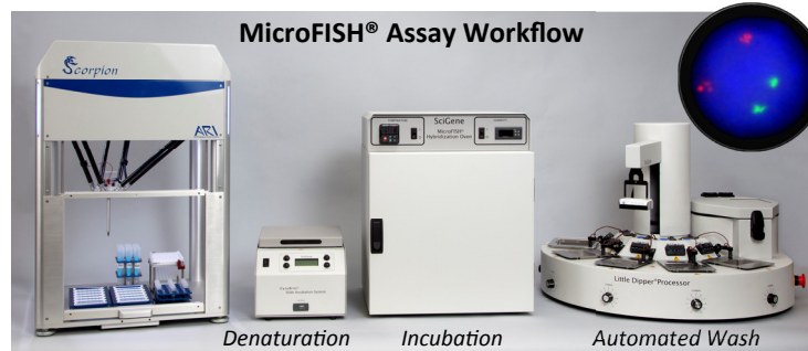
The Scorpion Robot dispenses fixed cells onto MicroFISH Slides for denaturation on the CytoBrite® PLUS, incubation in the MicroFISH Oven and wash on the Little Dipper Processor, ready for counterstaining and visualization.
