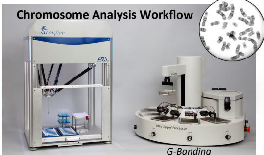
The Scorpion Robot dispenses metaphase cells onto microscope slides for G-Banding on the Little Dipper® Processor, ready for visualization.
