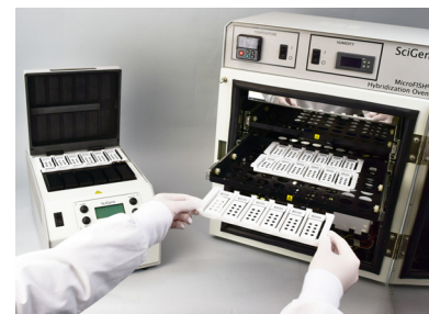
Denatured slides are transferred from the CytoBrite System to the MicroFISH Oven.
