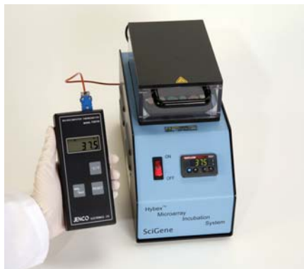
Calibration with a digital thermometer ensures accurate temperatures.
